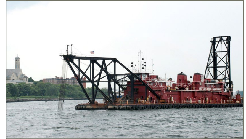
Cutter suction dredgers (CSDs) are classified as hydraulic dredgers – sand, clay, rock debris
